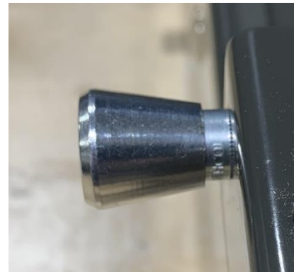
SPRING PLUNGER NOT RETRACTED
