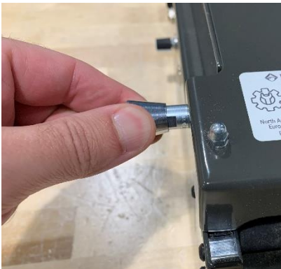
PULLING OUT SPRING PLUNGER
